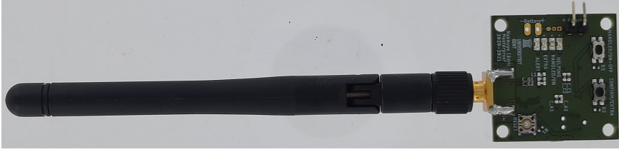
Figure B.5: The soldered PCB with the hinged dual-band Delta 7A from Siretta connected.
