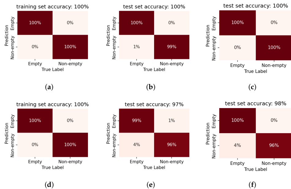
Figure 12. The confusion matrices of LPCC-based LR models on the data gathered from the tank wagon. Results are presented for the binary classification task, for prototype 1 (first row) by model 5 and prototype 2 (second row) by model 6. The first column indicates the performance on the training data, when only a single impulse is considered. The second column indicates the accuracy on the test set, again for a single impulse. The third column shows the benefit of fusion across three impulses. The trends are the same as in the case of the container experiments, with high accuracy after decision fusion. 100% accuracy is obtained by Prototype 1, installed at the bottom of the container. MFCC features yield poorer results—consistent with prior observations on container data—and are, therefore, not presented.
