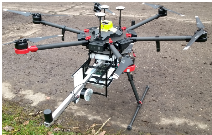
Fig. 7. The LiDAR mounted at \alpha = 88^\circ . This was achieved by 3D printing with an inclination of 2^\circ .
