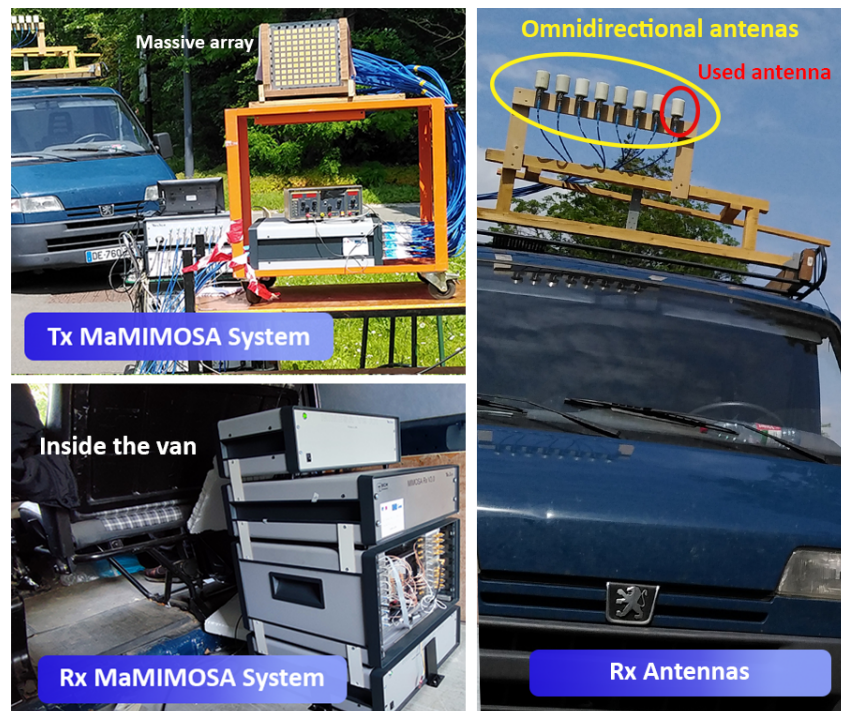
Figure 3. Montage of the Tx and Rx MaMIMOSA system showing the massive Tx array and Rx omnidirectional antenna.
