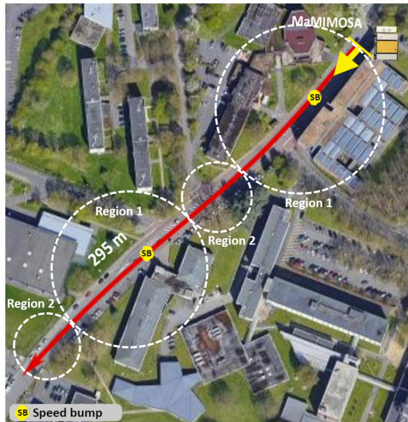
Figure 2. Top view of the V2I measurement campaign scenario at the University of Lille campus. The dashed circles indicate the two identified regions with distinct propagation characteristics.
