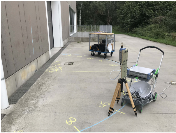
Fig. 2. Measurement setup for fiber cement reflection measurements with a 45^\circ incident angle.
