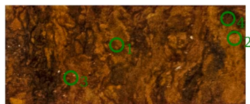
Fig. 8 RGB image of sample six. The green circles indicate the FTIR measurement location.
