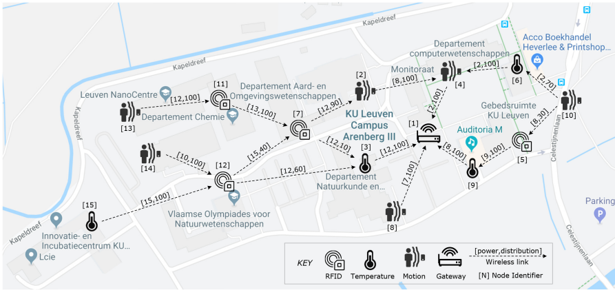
Fig. 1. DeltaIoT deployment at the KU Leuven campus (borrowed from Reference [69]). The gateway is marked by the blue icon in the center. The data collected by the sensors is sent over multiple wireless links to this gateway.
