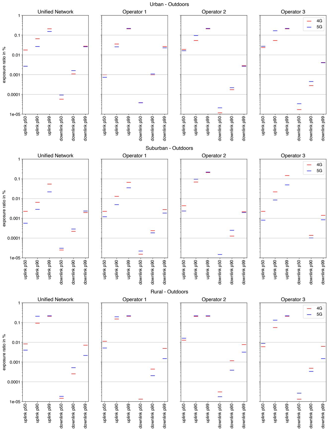
**Figure 5:** Uplink and downlink exposure ratios between different operators and a unified network in the three different environments for use case 1.
