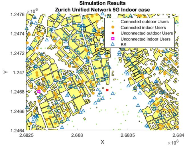
Figure 4: Use Case 1 intermediate result snapshot in Zurich city center.
