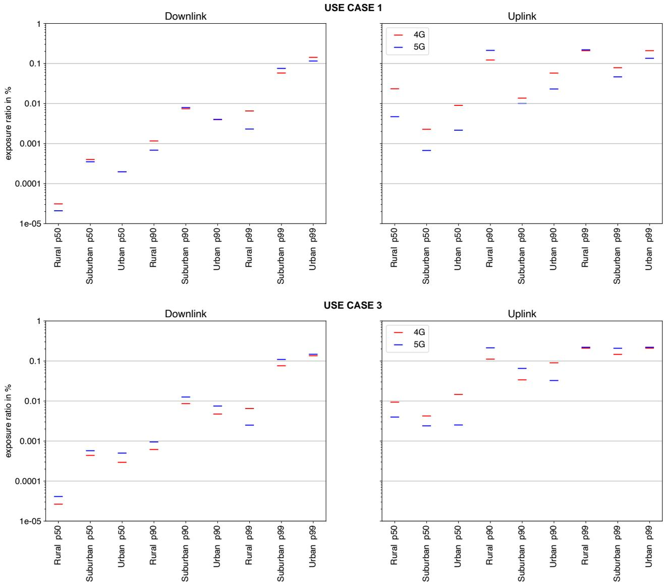
Figure 6: Downlink and uplink exposure ratios in different environments for use case 1 and use case 3 in the unified network.
