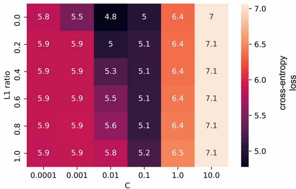
Figure 5 | Grid search over the hyperparameters of Elastic-Net logistic regression, using a calibrated hydraulic model for measurement campaign 1 ('MC1, calibrated'). The mean cross-entropy loss is computed over 9 experimental leaks.
