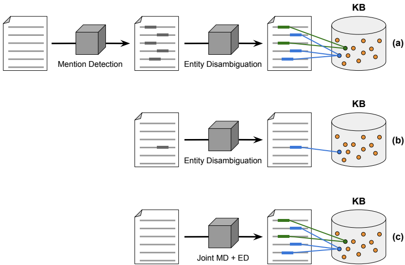
Figure 1.8: Figure showcasing an example of entity detection and entity disambiguation information extraction (IE) tasks in order to illustrate three IE learning setups: (a) pipelined setup where separate models are used sequentially for each of the tasks in order to produce the desired output given a plain document (i.e., without annotations) as input, (b) single task setup, where the ground truth annotations (i.e., mention(s) to disambiguate in the showcased example) are already given as input to the model, (c) end-to-end joint setup where a single model is trained and evaluated jointly on multiple tasks necessary to produce the desired output given a plain document as input.
