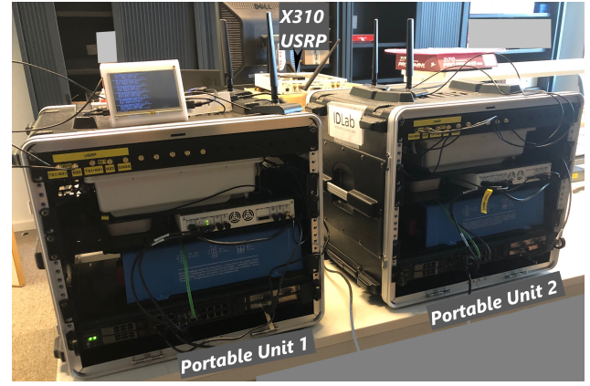
Figure 5: Setup used for LTE and 5G NR dataset collection.
