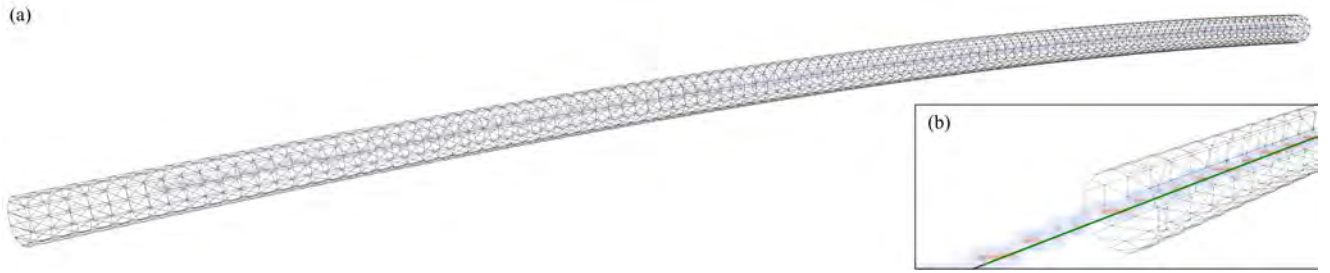
Figure 1: (a) Curve representing a fiber in 3d space and the voxels it was estimated from. A wire frame around the curve is shown to visualize the triangle mesh model of the fiber that is used in the end to represent the fiber for generating projections. (b) shows a close up of a part of the voxels (red and blue), center line (dark green) and the wire frame (black) is partially cut to reveal the voxels and center line.
