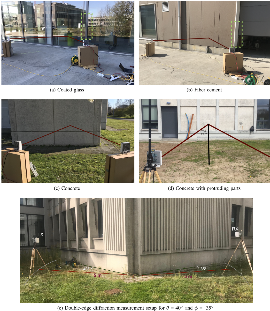
Figure 2. Building reflection and diffraction loss measurement setups.
