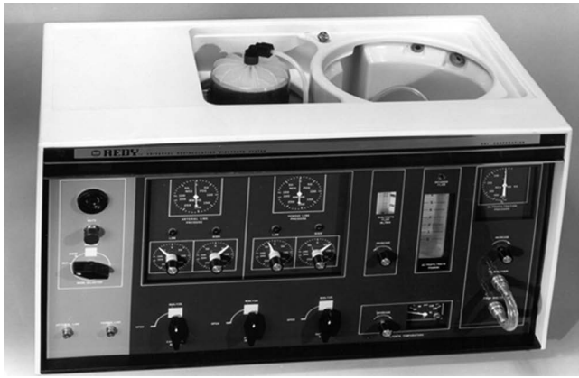
Figure 1. The URS SorbSystem (Redy) Dialysis Machine, with Sorb Column (middle, top) and 6L dialysate reservoir (ca 1979). 3
