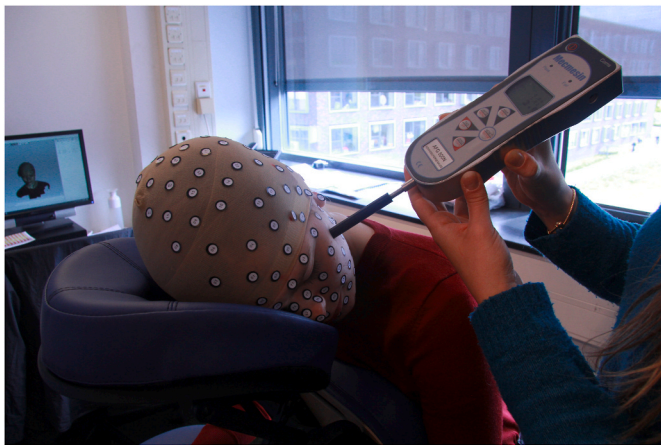
Fig. 1. Mecmesin AFG 500N pressure gauge with 3D printed PLA \varnothing 10 mm tip, and participant with EEG 10–20 landmark grid headcap and landmark stickers on the face, head and neck. Researcher gradually increasing pressure on a landmark with pressure gauge until the participant indicates the PDT has been reached.
