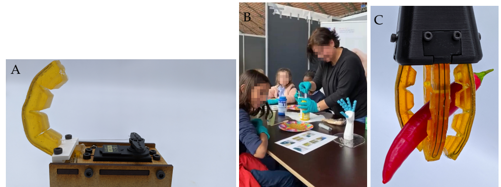
Figure 1. Result of the tutorial and workshop. (A): The self-healing soft finger with embedded sensor complete with the test set-up is the end goal of this tutorial. (B): The tutorial is easily adapted for use with commercial polymers, and can even be taught to children in an adapted version. No sensor was embedded in this case, and actuation was done manually. (C): The fingers made during the tutorial can for example be used in a gripper to pick up fruits.
