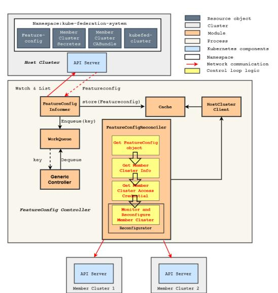
Figure 8. Architecture of the controller.
