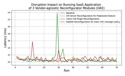
Figure 11. Disruption impact of the three Reconfigurator modules on SaaS application.
