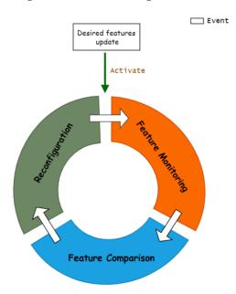
Figure 7. Feature compatibility controller's control loop.
