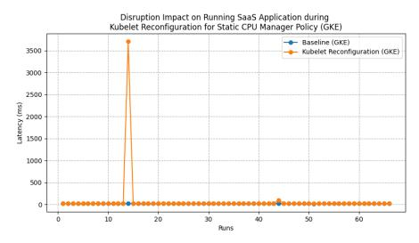
**Figure 14.** Disruption Impact on SaaS application (During Kubelet restart, no traffic routed to the Application).
