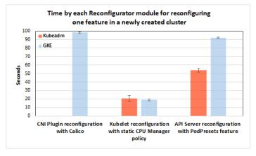
Figure 15. Reconfiguration time for each feature in a newly created cluster.
