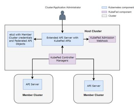
Figure 2. Cluster Federation based on KubeFed V2.
