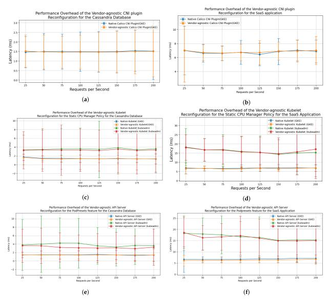
**Figure 9.** Performance overhead of the three Reconfigurator modules of the autonomic controller in comparison with native configuration using proprietary customization interfaces of two K8s vendors (GKE and kubeadm). An explanation for each subfigure (**a**–**f**) is given above it.
