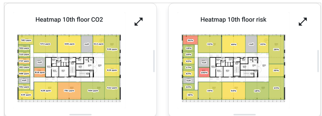
Figure 5. Heatmap visualization of the CO 2 concentration and COVID-19 aerosol transmission risk estimation of the 10th floor of our office building.
