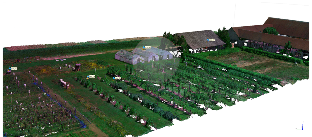
Figure 14. The resulting multispectral point cloud from the Bottelare dataset, here colored using the bands corresponding with the red, green, and blue wavelengths.
