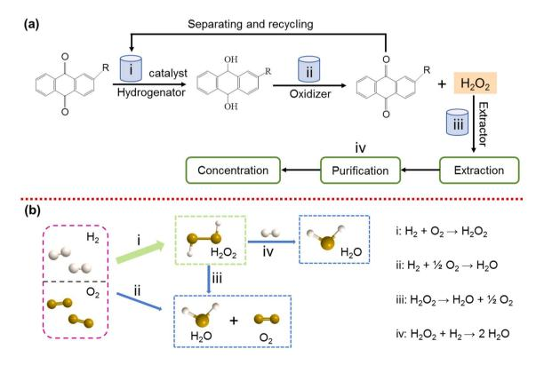
Fig. 1 Schematic illustration of **a** the anthraquinone (AQ) oxidation process and **b** the direct synthesis from  $H_2$  and  $O_2$
