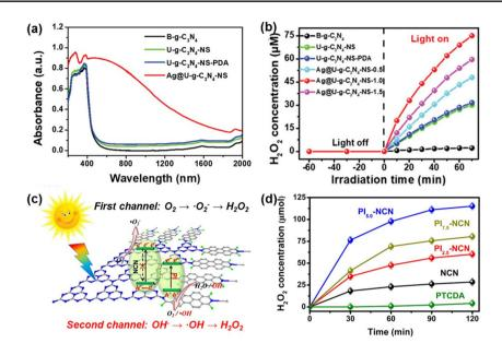
**Fig. 4** a UV-DRS absorption spectra of different samples. b  $H_2O_2$  concentration of different catalysts. Reproduced with permission from Ref. [91]. Copyright 2019 Wiley–VCH Verlag GmbH & Co. KGaA, Weinheim. c Proposed mechanism of different sites on all-solid-state Z-scheme heterojunctions for photocatalytic production of  $H_2O_2$ . d Concentration of generated  $H_2O_2$  in NCN and PIx-NCN systems. Reproduced with permission from Ref. [97]. Copyright 2017 Elsevier
