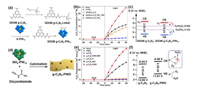
**Fig. 5** a, d Schematic illustration of the synthetic route to 3DOM  $g-C_3N_4-PW_{11}$  and  $g-C_3N_4-PWO$ . b, e  $H_2O_2$  production over different catalysts in 60 min. c, f Scheme of energy levels and charge transfer pathways of 3DOM  $g-C_3N_4$  and 3DOM  $g-C_3N_4-PW_{11}$ ,  $g-C_3N_4$  and  $g-C_3N_4-PWO$ . Reproduced with permission from Refs. [105, 107]. Copyright 2017 Elsevier and 2018 Elsevier
