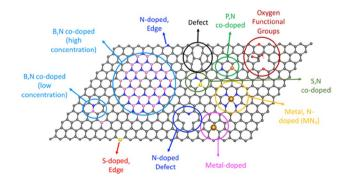
Fig. 13 Schematic demonstration of tuning electronic structures of carbon electrocatalysts for electrocatalytic  $H_2O_2$  production via the 2e<sup>-</sup> ORR pathway. Reproduced with permission from Ref. [18]. Copyright 2020 American Chemical Society
