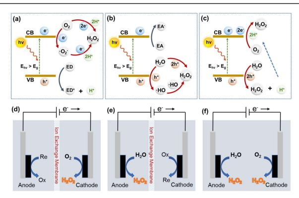
Fig. 2 Simplified schematic of photocatalytic  $H_2O_2$  generation from **a** ORR, **b** WOR and **c** dual-channel pathway. Simplified schematic of electrocatalytic  $H_2O_2$  production from **d** ORR, **e** WOR and **f** dual-channel pathway
