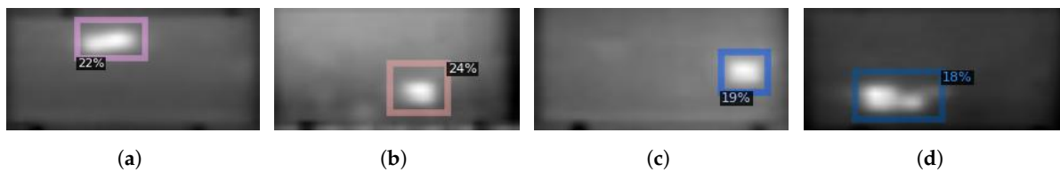
Figure 10. Four different hotspots (a–d) detected using our region-based CNN algorithm on the dataset acquired at Serramanna, Italy.
