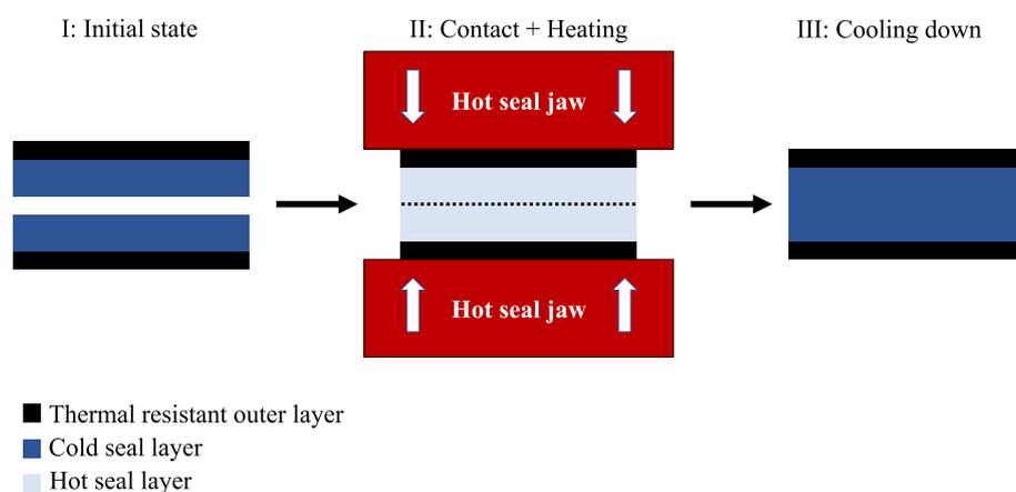
**FIGURE 1** Three basic steps of a heat seal process with hot jaws; figure adapted with permission from Ilhan (2021).<sup>4</sup>
