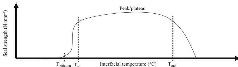
FIGURE 2 Temperature dependence of seal strength of PE.
