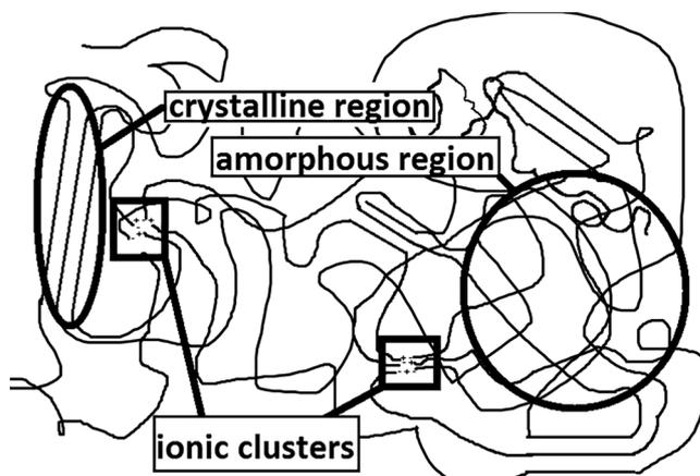
FIGURE 4 Schematic structure of different regions in ionomers.
