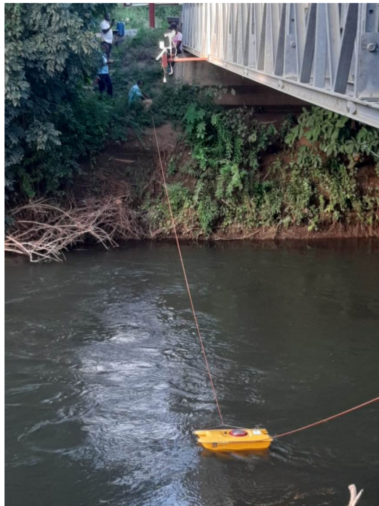
Figure 6. Echo sounding technique employed to determine initial river level.
