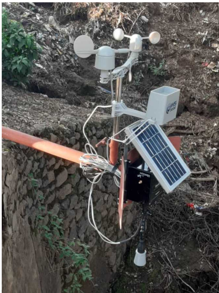
Figure 4. Plug&Sense! Smart Agriculture PRO with all parts connected.
