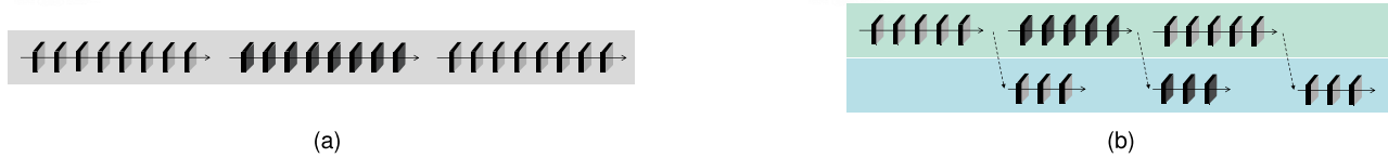
FIGURE 3. Network workload distribution for single- and two-stage approaches. CNN classification over three frames is shown for (a) single-stage execution on a particular hardware, or (b) two-stage concurrent execution on two hardware devices.
