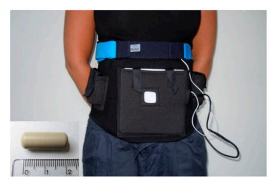
**Figure 2.** WIC, sensor array and receiver system presented by Motilis Medica when moving to an AC magnetic localization method [50] from their previous approach of using a permanent magnet within the WIC.
