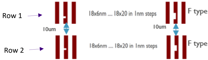
Defect Type F9 on mask Defect Type F9 on row 1 Die (1,0) Defect Type F9 on row 2 Die (1,0)
