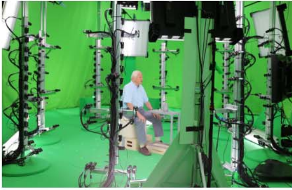
Fig. 17. Camera setup by Sky Studios, used to create a VR experience in the National History Museum in London, UK [120]. More than 100 depth cameras were used to create volumetric video.
