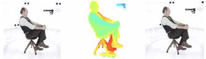
Fig. 19. Example of a dense depth map calculated per frame for each stereo camera pair.
