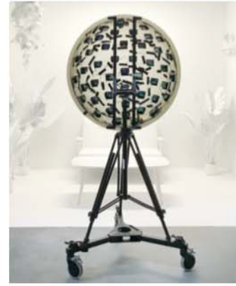
Fig. 28. Illustration of the light field capture rig proposed by Broxton et al. [28].
