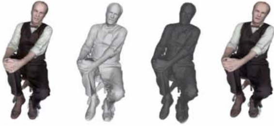
Fig. 20. Example of the resulting point cloud and 3D models such as meshing, simplification, and texturing (from second left to right).
