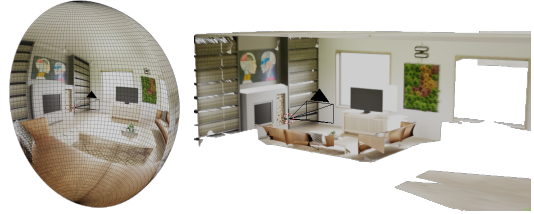
Fig. 1. Left: (Half of) a 360° image is shown to a viewer wearing a VR headset. In essence, the image is projected on a sphere which remains stationary with respect to the viewer’s head. There is no motion parallax. Right: Depth information about the original scene is added. The geometry does not move together with the viewer, resulting in the correct depth perception.
