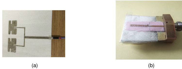
Fig. 3. Textile antenna arrays: (a) 2x1 patch antenna array operating at 2.45 GHz (image taken from [25]). (b) Yagi-Uda antenna operating at 60 GHz (image taken from [61]).
