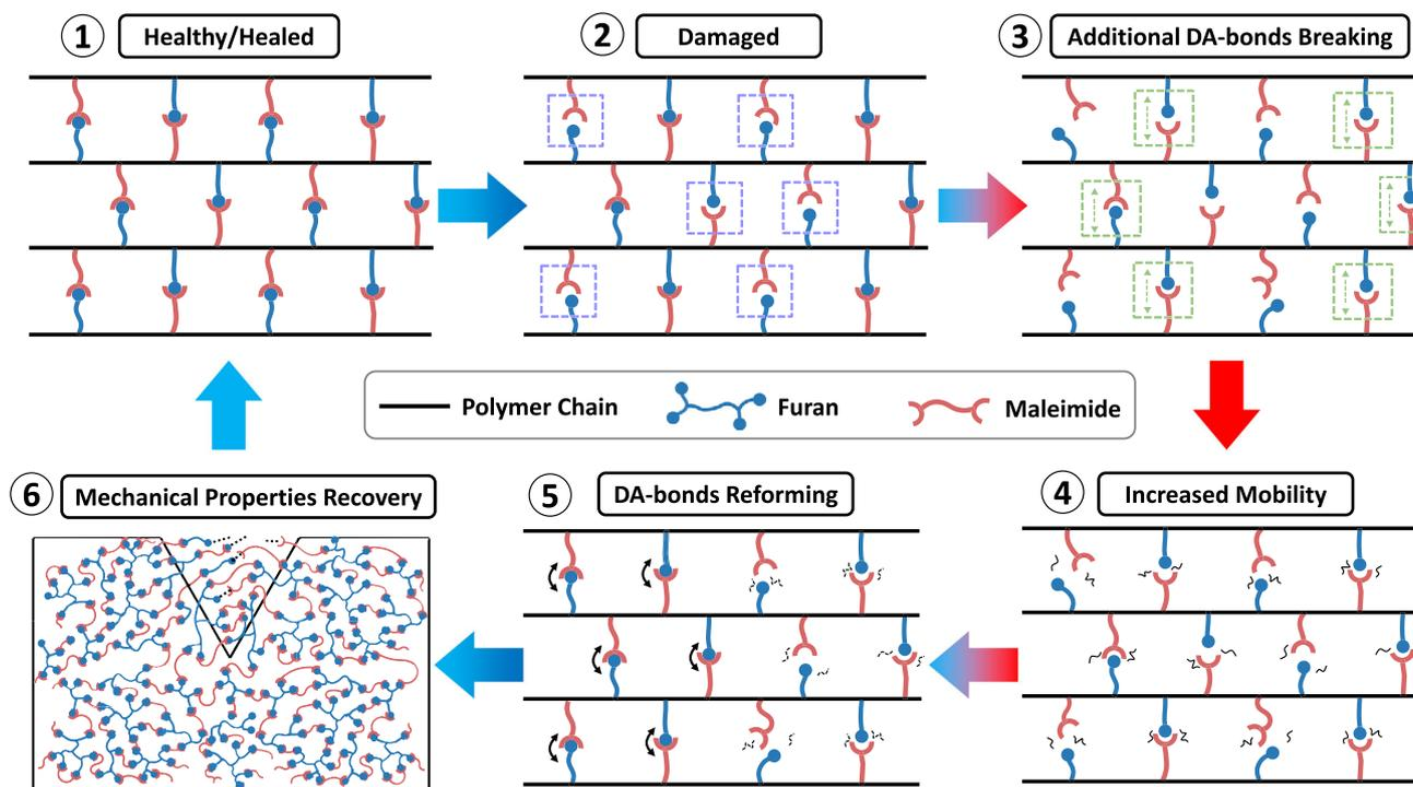
**Figure 10.** The self-healing heat-cool cycle of the DA polymer and the accompanying illustrations of the DA reversible process.
