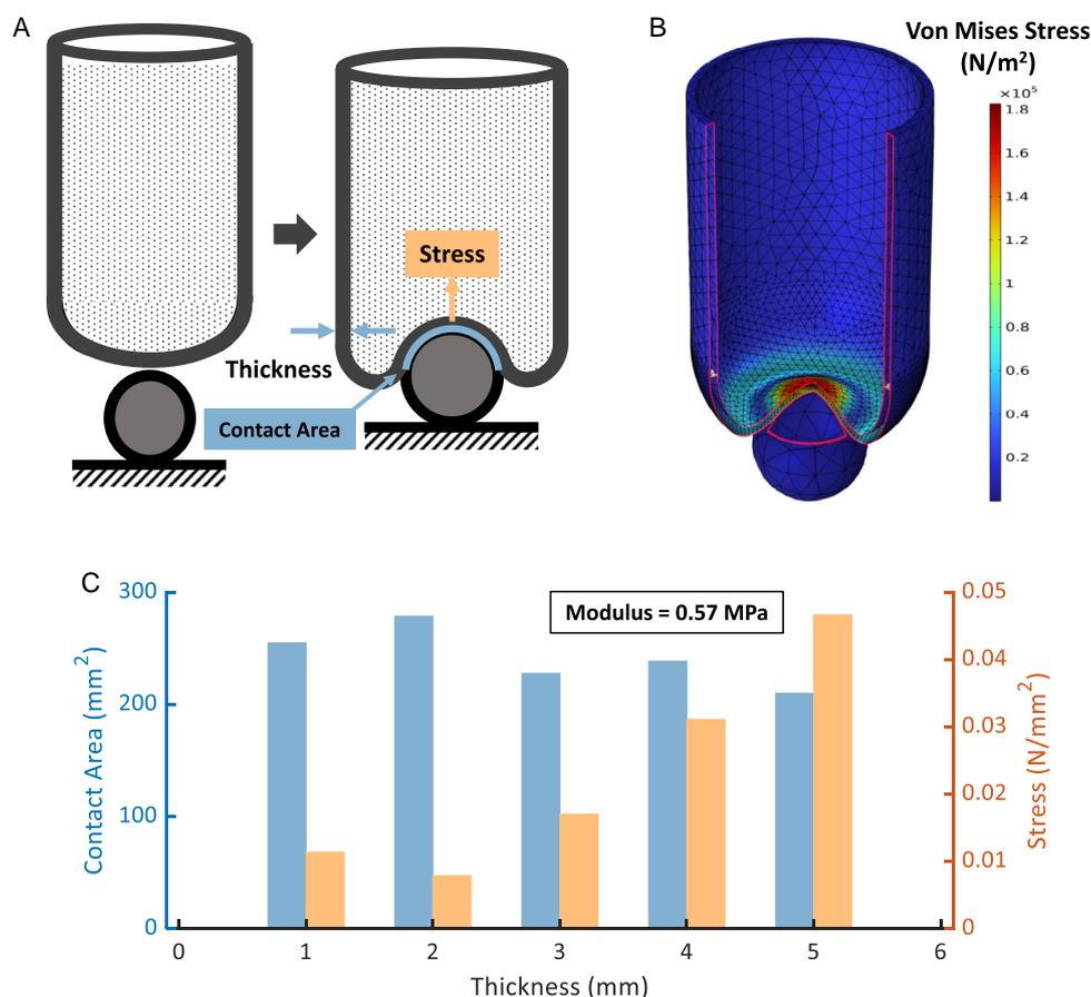
**Figure 3.** The FEA-based morphological optimization. A) Schematic of adaptive grasping, where the contact area and stress play key roles in the grasping performance. B) Cross-section view of an FEA simulation of the deformation in the SHUG upon adaptation to a spherical object with a diameter of 25 mm. C) The contact area and the stress as a function of the cover thickness for a fixed elasticity modulus of 0.57 MPa.
