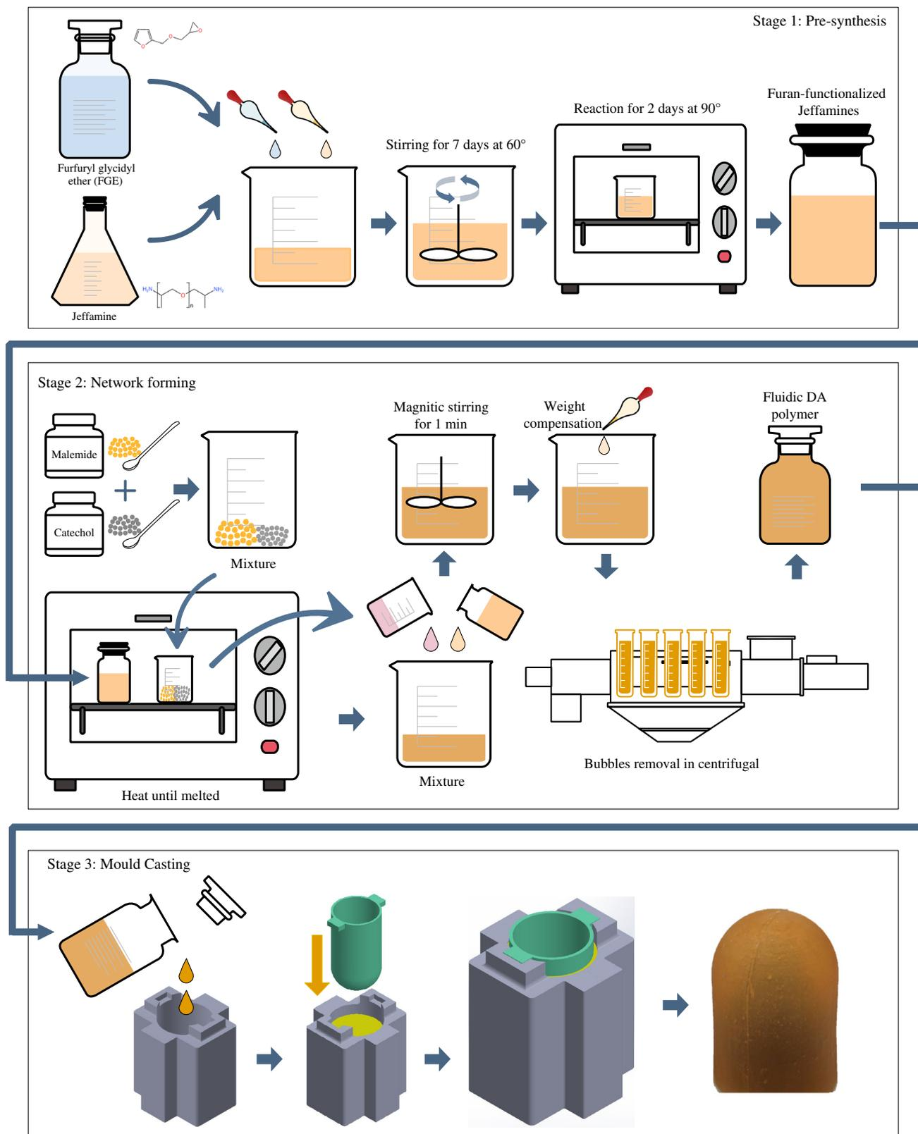
**Figure 11.** Flowchart of the fabrication of the self-healing membrane.
