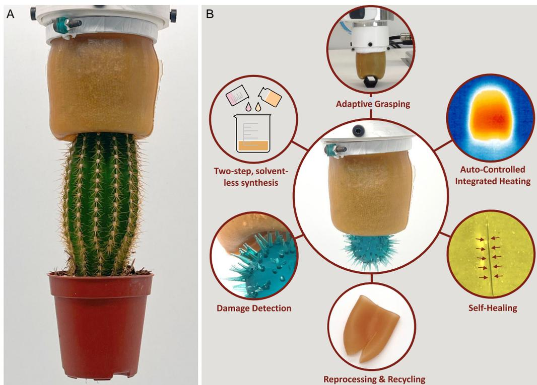
**Figure 1.** A) SHUG is adaptively grasping a hazardous object (cactus) and B) the highlights of the integrated system.
