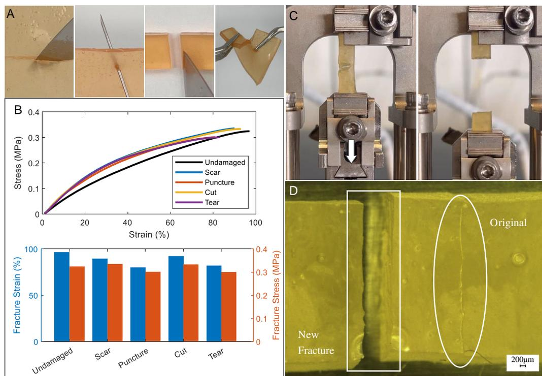
**Figure 8.** The DA membrane is able to self-heal from various macroscopic damages. A) Four types of damages including (left to right) scratch, puncture, cut, and tear. B) The comparison of stress–strain curve and elongation rate for the DPBM-FT3000-R05 sample before and after the self-healing. C) The axial normal stress and strain measurement in a tension test. D) For a healed sample, the original damaged part is no longer a weak point.
