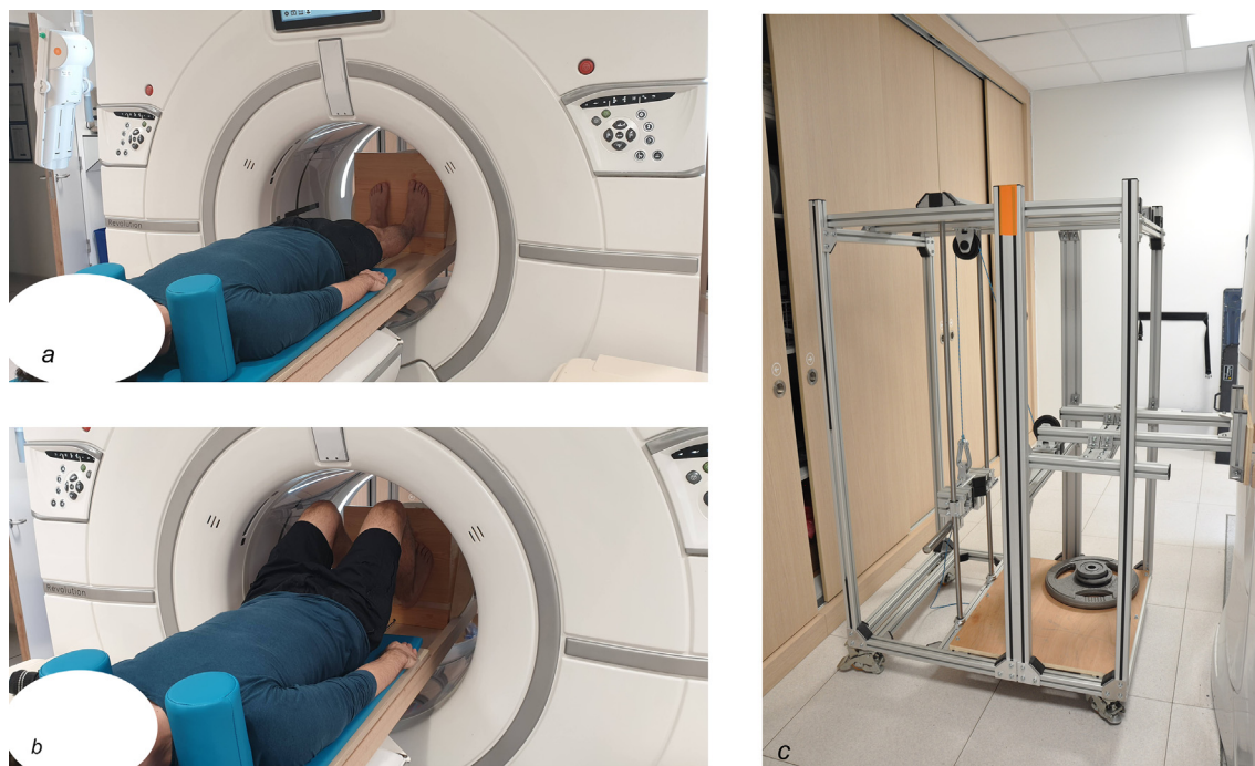
Figure 2. Knee in fully extended position (a), and maximum knee flexion achieved (b), counter-weight system (c).
