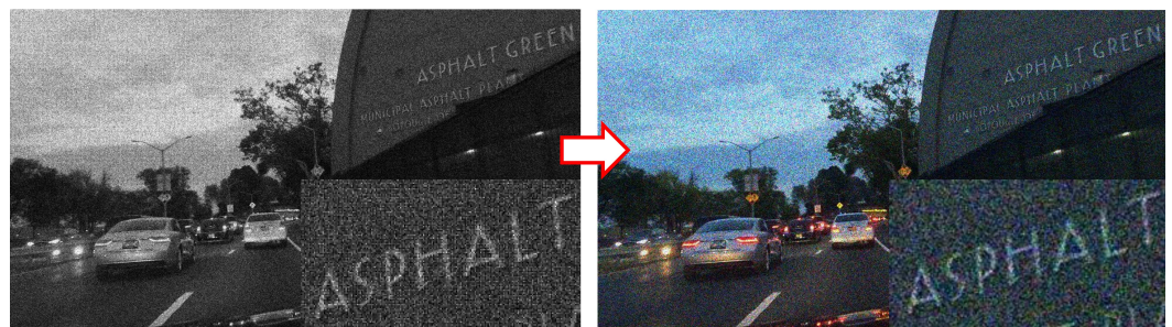
Figure 7. The appearance of noise with demosaicing and noise artifacts when the noise is applied before demosaicing, as happens in reality. Left: Bayer CFA mosaiced image with noise with Poisson distribution. Right: the image on the left demosaiced with the algorithm presented in [56]. Note the complex structure and the severity of the noise artifacts in the demosaiced image. After demosaicing, the noise appears with a more complex structure than the initial Poisson distribution in the mosaiced image. It is color correlated and it is dependent on the local spatial activity of the image content.
