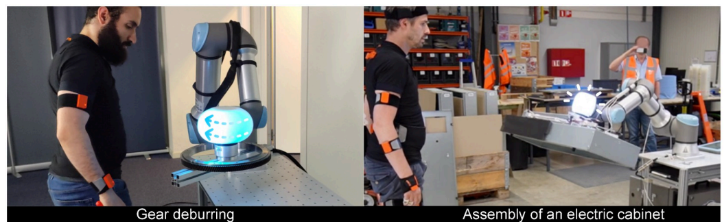
Fig 5. Customised versions of Antropo with the Universal Robots UR16e: Gear deburring (left) and assembly of an electric cabinet (right).
