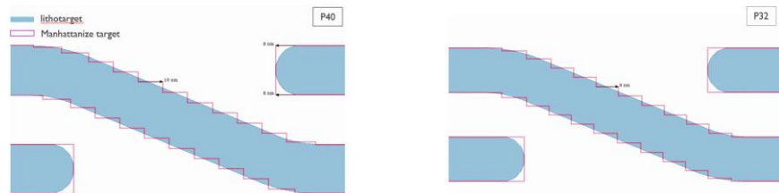
Figure 10. Manhattanized target with 10nm step-size for P40 (left) and 8nm step-size for P32 (right)
