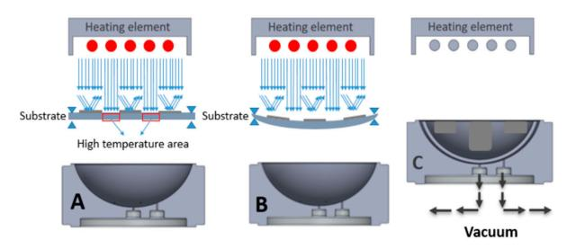
**Figure 20.** The effects of printing a reflective layer on the substrate on light absorption in the thermoforming process. (**A**) Heating process, (**B**) Starting the vacuum, (**C**) Thermoforming.
