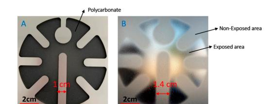
**Figure 3.** (**A**) The heat-blocking mask made in aluminum, (**B**) polycarbonate which has been exposed to IR radiation.
