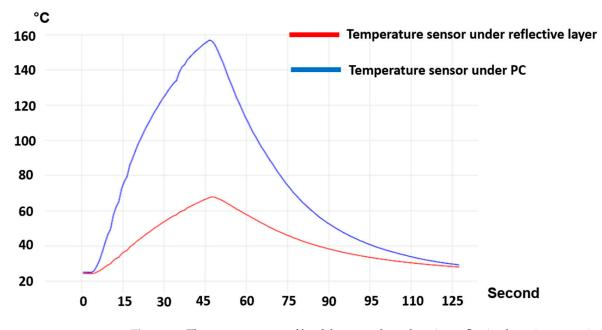
**Figure 19.** The temperature profile of the area where there is a reflective layer in comparison with the area where there is no reflective layer.
