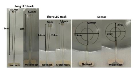
**Figure 8.** Measurement results of the thermoformed sample using a 60% elongation mold. When "No-mask" is mentioned, it means we have not used any mask to restrict the heat over the substrate in the thermoforming machine and "Metal mask" means we have used a specific mask, which is depicted in Figure 4B, to restrict the exposure of the substrate.
