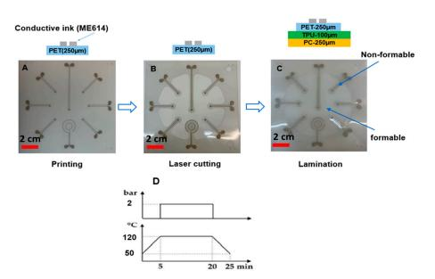
**Figure 12.** (**A**) Printing the conductive track on PET by using screen printing. (**B**) Laser cutting the printed sample to make the non-stretchable parts. (**C**) Lamination of the PET substrate with polycarbonate and TPU to make a thermoformable stack. (**D**) The lamination profile.
