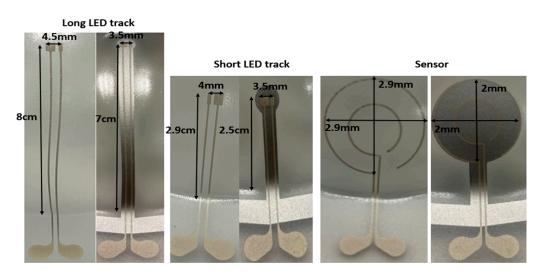
**Figure 23.** Measurement results of the thermoformed samples (for 3 different designs) using a 60% elongation mold. Comparison between the thermoformed samples with (right-hand picture for each design) and without (left-hand picture for each design) a reflective layer. Measured lengths are listed in Table 3.
