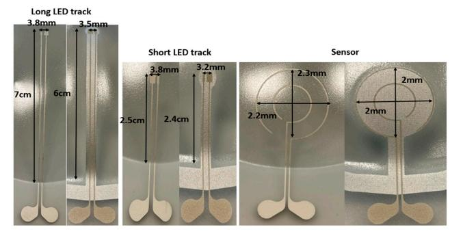
**Figure 24.** Measurement results of the thermoformed sample using a 16% elongation mold. Comparison between the thermoformed samples with and without a reflective layer.
