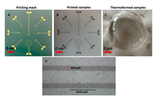
**Figure 6.** (**A**) Screen mask. (**B**) Printing result on the polycarbonate substrate using ME614 as the conductive ink. (**C**) Thermoforming result by using a semi-sphere mold with 60% elongation. (**D**) detailed view of 2 printed tracks (darker grey) after thermoforming.
