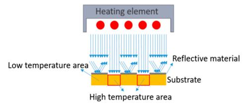
Figure 15. A substrate with a printed-reflective layer and temperate difference in the substrate.
