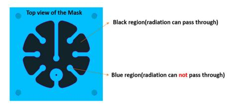
**Figure 2.** The blue region represents the area that IR radiation cannot penetrate, and the black area shows the areas exposed to IR radiation.
