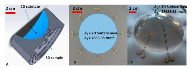
**Figure 7.** (**A**) A cross-sectional view of the 2D substrate and 3D sample surface area. (**B**) The 2D surface region in the substrate that is heated and formed. (**C**) The 3D surface area after thermoforming.
