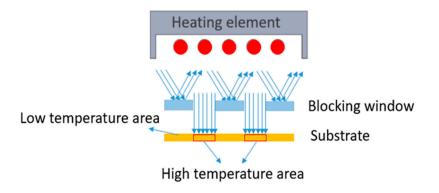
Figure 1. Using a blocking window to restrict the heat in the thermoforming machine.
