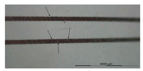
**Figure 10.** Micro crack formation as the result of the stretch of the ink during thermoforming by using a 60% mold elongation.
