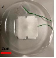
Thermocouple installation to the substrate in the thermoforming machine
