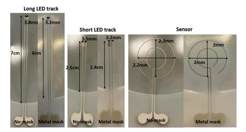
**Figure 9.** Measurement results of the thermoformed sample using 16% elongation mold. "No-mask" means we have not used any mask in the thermoforming machine to restrict the heat over the substrate and "Metal mask" means we have used a specific mask, which is depicted in Figure 10, to restrict the exposure of the heat to the substrate.
