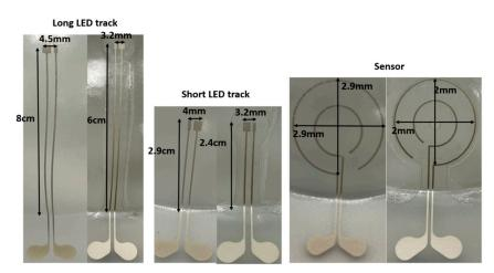
**Figure 14.** Measurement results of the thermoformed sample using a 60% elongation mold. Comparison between the typical fabrication process (the typical fabrication process is actually the "No mask" production process of the heat-mask methodology) and our proposed approach to fabricating in-mold electronics.
