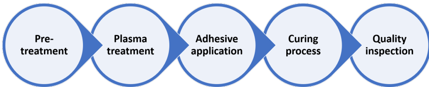
Fig. 2: Schematic overview of the adhesive bonding process
