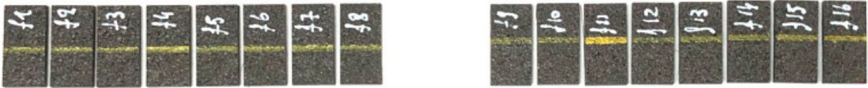
Figure A11. ILSS test coupons with 80/120 \mu\text{m} fiber embedded along the yellow line.
