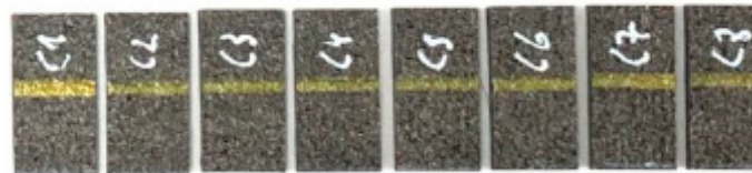
Figure A13. ILSS test coupons with 106/160 μm fiber embedded along the yellow line.
