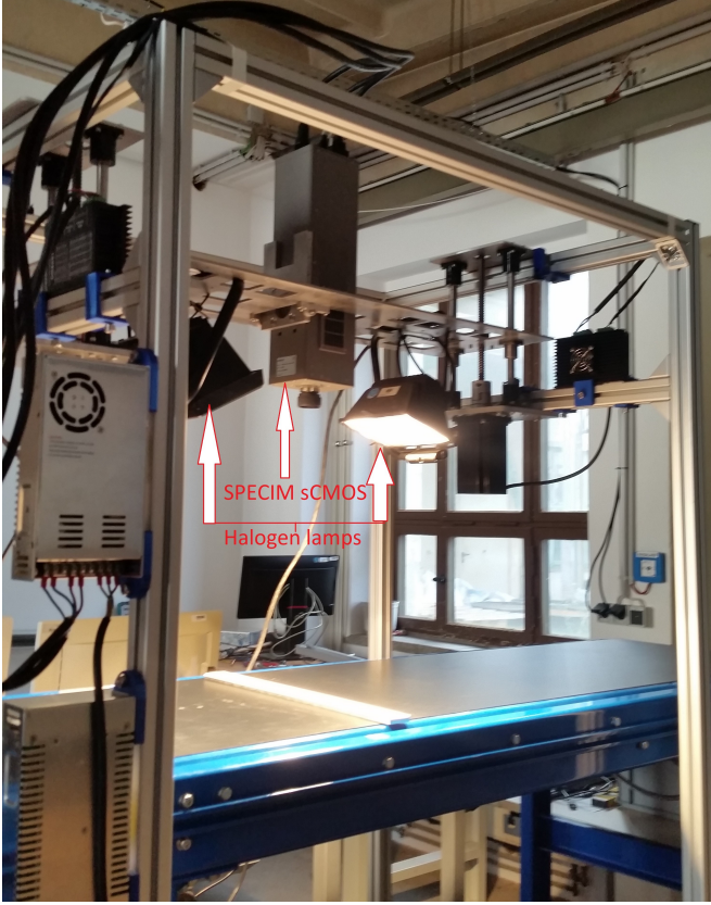
Fig. 4: Conveyor belt scanner with the Specim sCMOS camera mounted on it.
