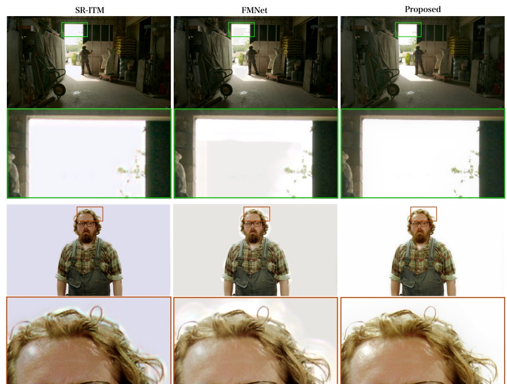
Figure 11. Sample frames illustrating artifacts in highly saturated regions, with visible distortions generated by the SR-ITM and FMNet methods. These artifacts become more noticeable when the video sequences are displayed on the SIM2 HDR screen. Images have been tone-mapped for presentation.
