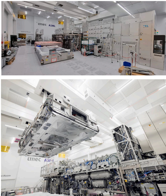
Fig. 10. Step by step assembly (Top picture: wafer stage, bottom picture: reticle stage) of a High NA EUV tool in joint imec-ASML High-NA lab at ASML's headquarters in Veldhoven (NL). Credit: ASML.
