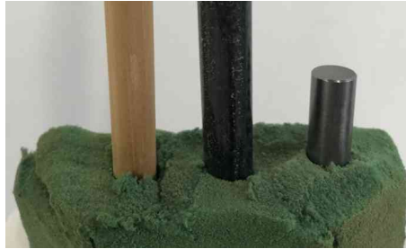
Fig. 4. The scanned multiple cylinders sample. Materials from left to right: wood, carbon (hollow), beryllium.
