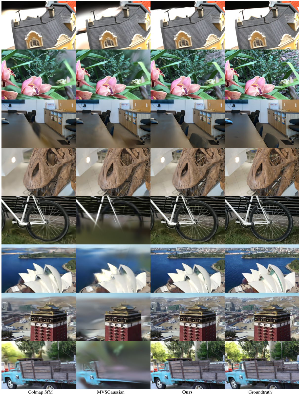
FIGURE 3. A comparison of three splat initialization methods. The results shown are (closeup) renders after 1000 3DGS training iterations.
