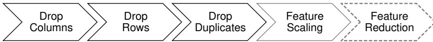
Figure 2.2: The preprocessing pipeline consisting of five steps of which the last one is not employed for the algorithms relying on a reconstruction error as anomaly score.
