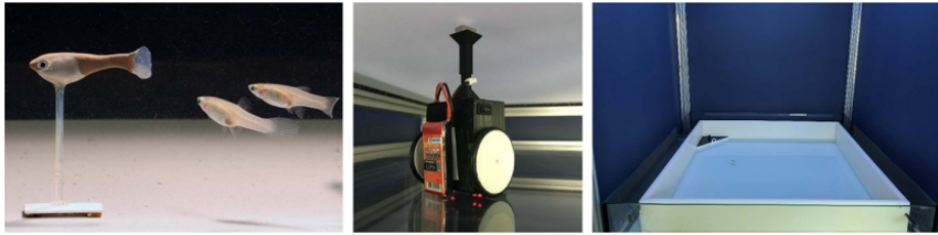
Figure 5.1: Figure reproduced from Maxeiner et al. [31] with permission, showcasing the RoboFish system. Left panel; a 3D-printed fish replica is attached to a magnetic base, which aligns with the robot. Hence the replica can be moved directly by the robot at constant height. Center panel; a wheeled differential-drive robot moves on a transparent platform below the test tank, carrying a neodymium magnet. Right panel; the tank is a quadratic ( 1\text{ m} \times 1\text{ m} ) with a triangular start box used as shelter for the live fish at the beginning of each experiment.
