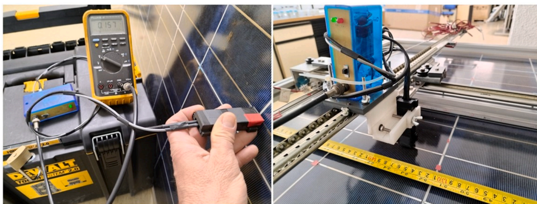
Fig. 1. On the left, the AMR sensor, its electronics and multimeter for recording the voltage output generated by the ribbon of a solar module, used as a portable device for detecting simple interruptions. On the right, the same sensor mounted on an XY frame with manual movement on the XY axes, placed on a solar module to record the magnetic signal along a ribbon of the module.
