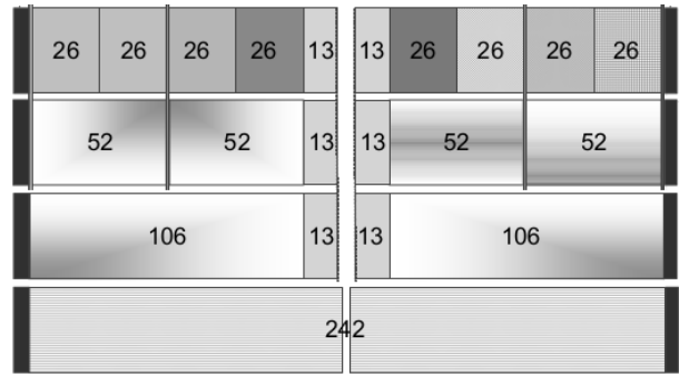
Fig. 1. IEEE 802.11ax RU locations for 20 MHz (adapted from [18]).
