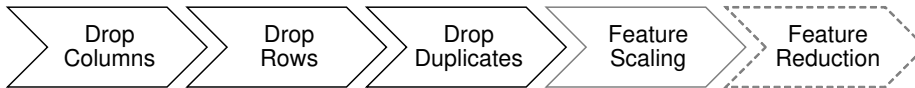
Fig. 2: The preprocessing pipeline consisting of five steps of which the last one is not employed for the algorithms relying on a reconstruction error as anomaly score.
