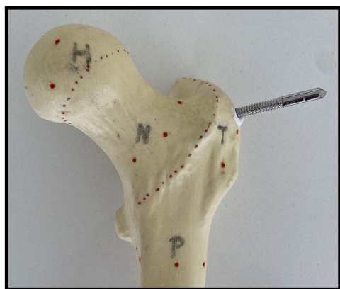
FIGURE 1 | Plastic femur replica with the four regions: H = head, N = neck, P = proximal T = trochanter. Each was marked with four holes of 1 mm diameter. The delineated area indicates the bony surface of the hip that would be visible during a surgical procedure, in this case, through an anterior approach. The pin in the greater trochanter was used to fix the reference IR reflective tracker.
