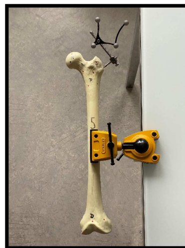
FIGURE 2 | Superior view of a plastic femur replica mimicking the anterior approach of the hip. A Steinman pin was drilled in the greater trochanter region to fix the IR reference tracker.
