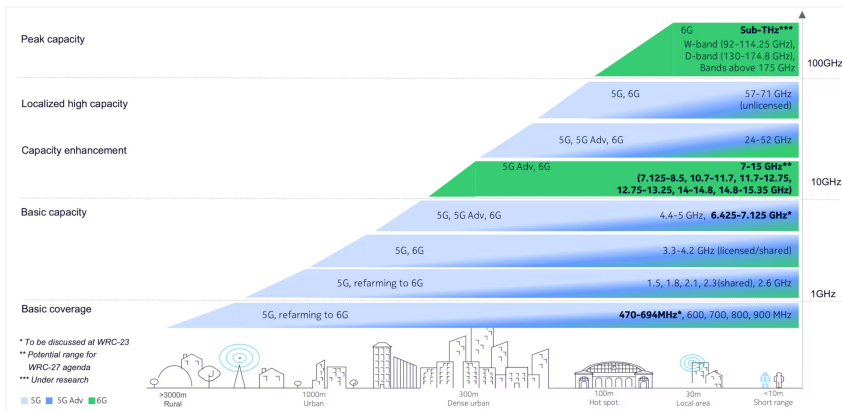
Figure 1.2: The 6G spectrum vision of Nokia [12]. Several new frequency bands are introduced, each serving their own specific area size with their envisioned total capacity requirement.
